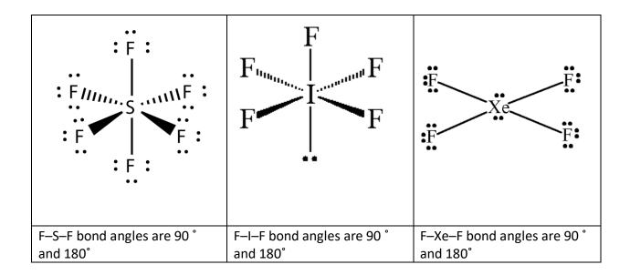
How do nonbonding (lone pair—LP) electrons explain the molecular geometries of  $F_4Xe$  and  $F_5I$ ? It makes no difference which bonding pair of electrons is replaced with a nonbonding pair, the resulting square pyramidal molecular geometry is the same for  $F_5I$ . However in the case of  $F_4Xe$  the nonbonding pairs must go 180  $^\circ$  apart to reduce the LP-BP repulsions.
